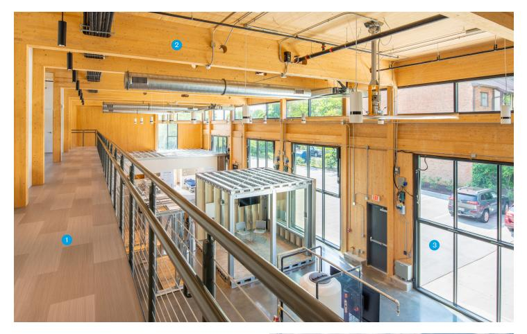
Innovative Recycled Materials Among the many sustainable applications used at ColLab, the 800 sq.-ft. catwalk is made from over 13,000 plastic bottles—the first commercial installation of this type of flooring.
