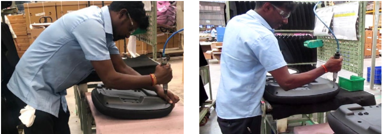
Before: The member had to bend in order to perform the seat cover assembly operation, causing fatigue in their spine. After: The height of the table was increased by 250mm to eliminate this operator fatigue.
